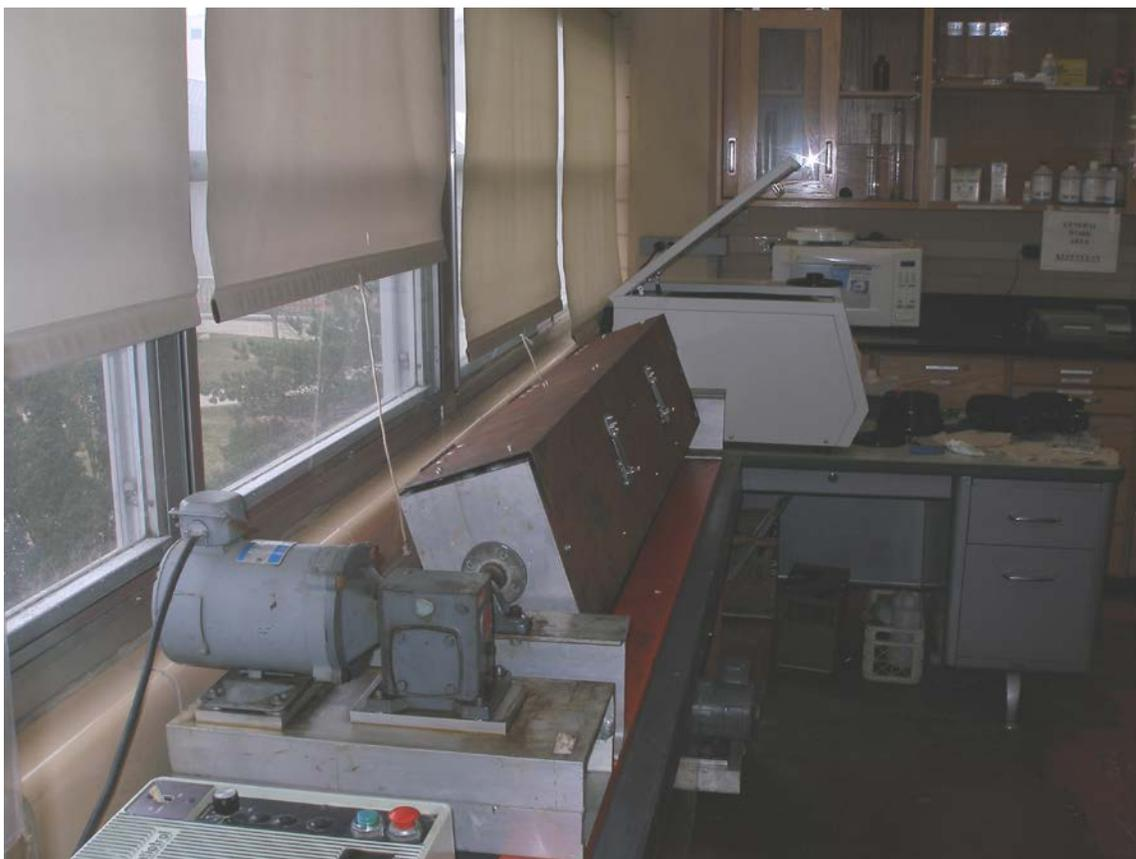
Fig. A2-11. Water leach test rotator.
