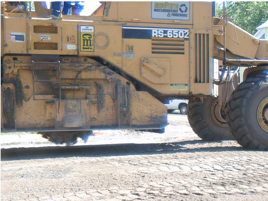
Fig. A1-5. Mid-section of road-reclaimer showing tines used to blend fly ash, water, and RPM.
