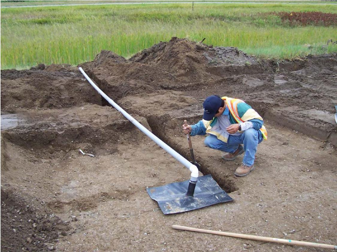
Fig. A2-2. Preparing drainage pipe from lysimeter to collection tank.
