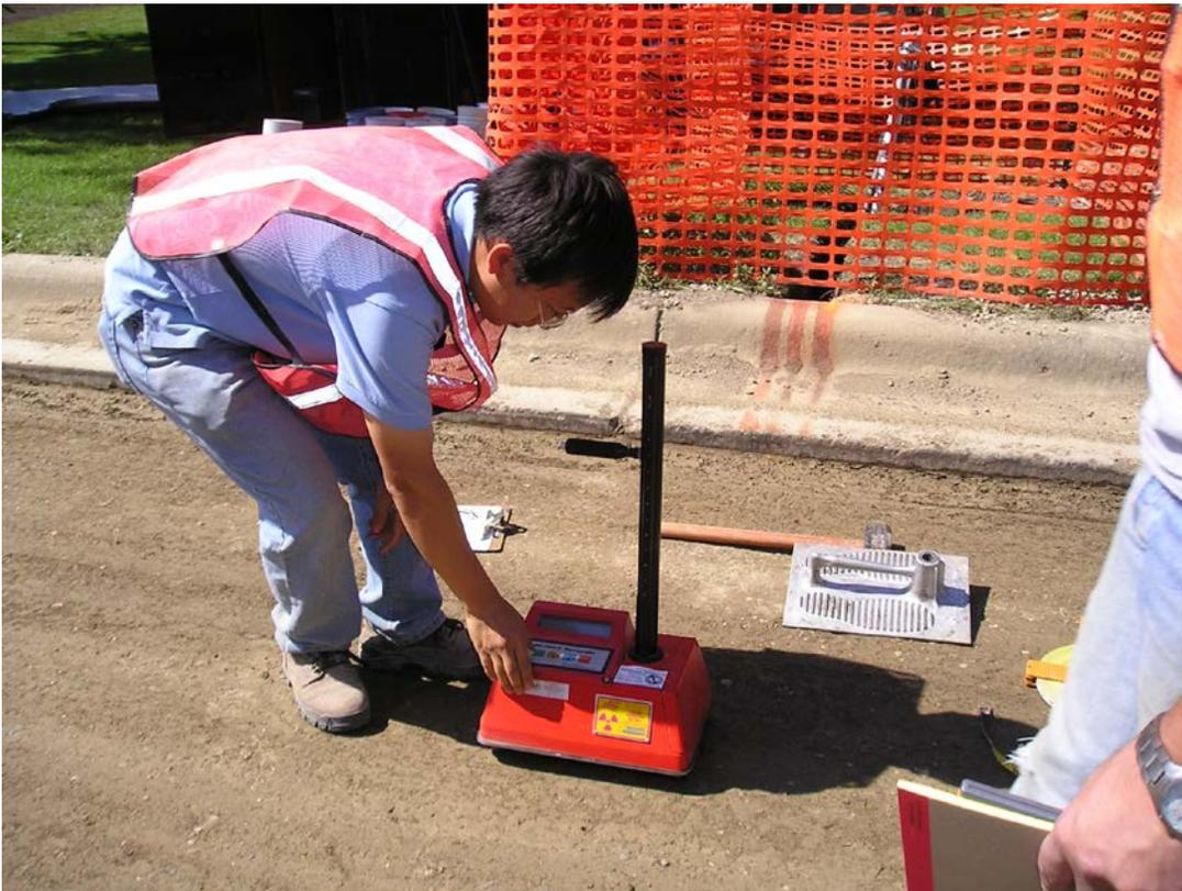
Fig. A1-6. Measuring water content and unit weight of stabilized RPM after compaction.
