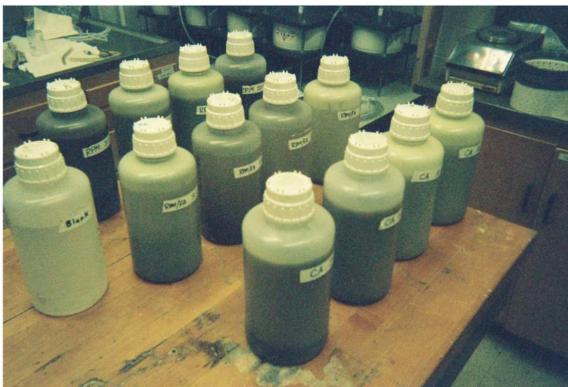
Fig. A2-12. MnROAD water leach test samples immediately after rotation.
