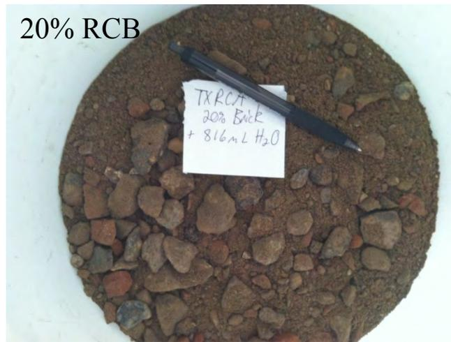
**Figure 9.18 0%, 10%, and 20%, RCB with TX RCA at OMC**
