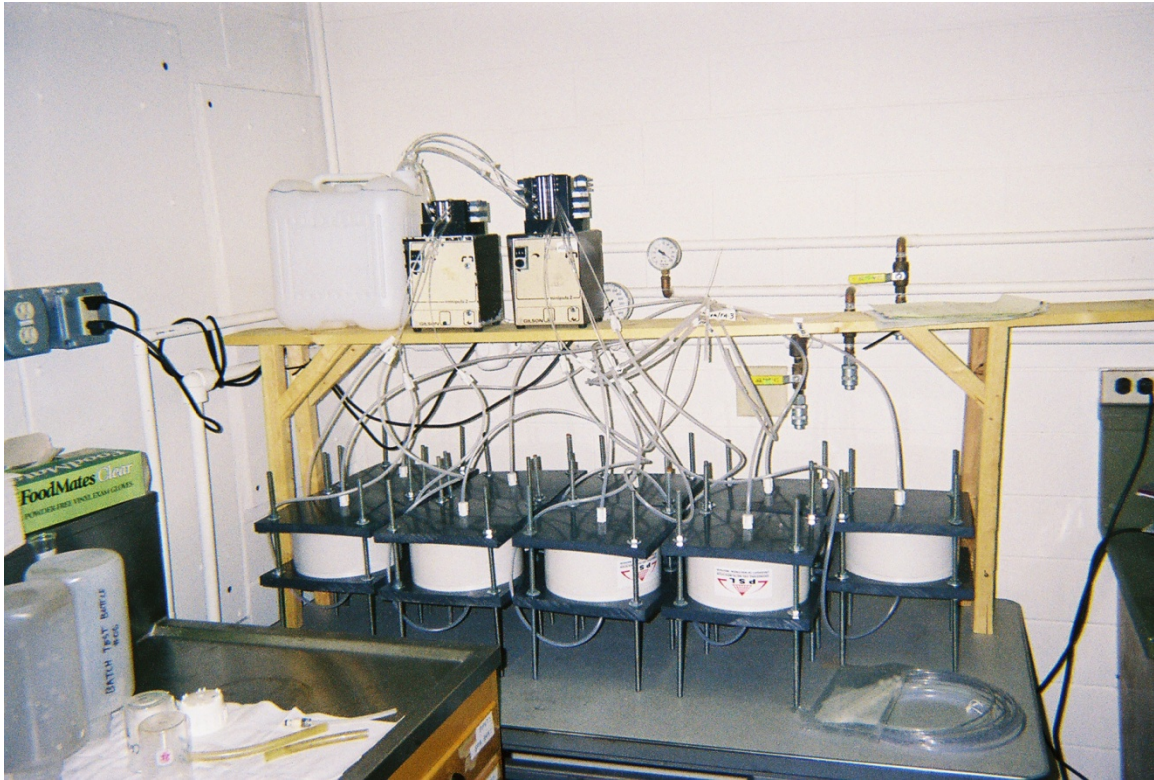
Figure A-10: Column leach test on MnROAD materials.
