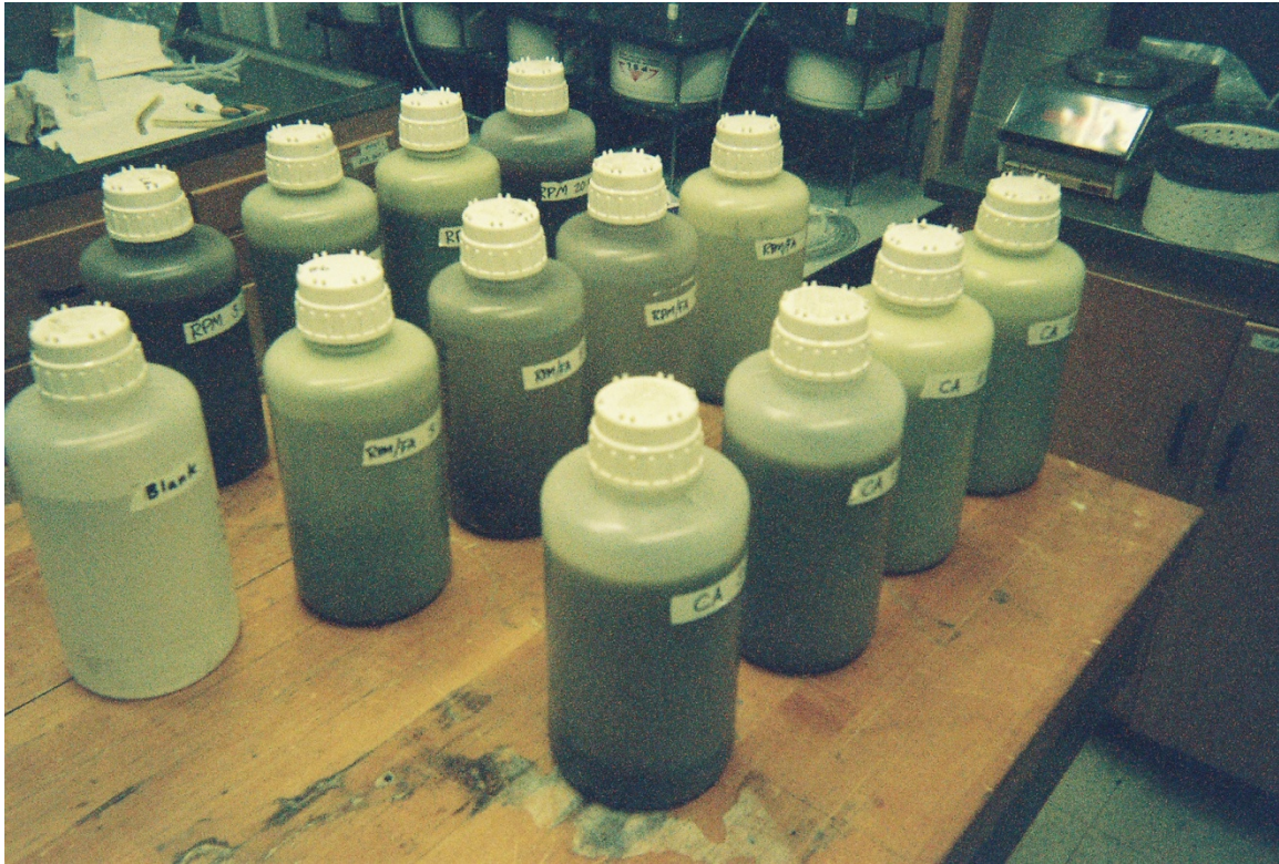
Figure A-12: MnROAD water leach test samples immediately after rotation.
