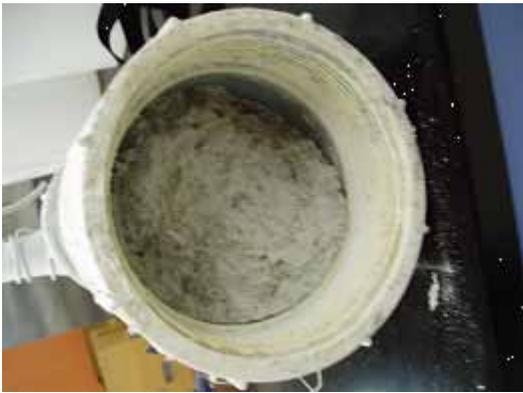
Figure 7. Less than 9.5 mm graded LFC material immediately after exposure to 10 F/T cycles (note consolidation of the material).
