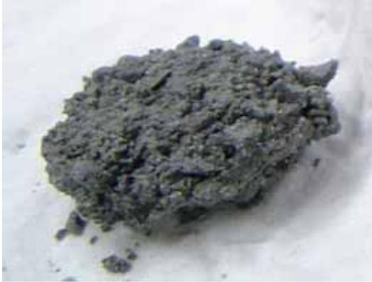
Figure 9. Less than 9.5 mm graded LFC material after exposure to 10F/T cycles and column leaching for 25 days (note aggregation of the concrete particles).
