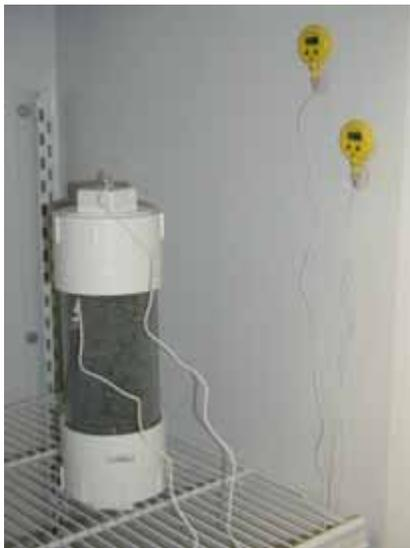
Figure 1. Column filled with LFC material during freezing.
