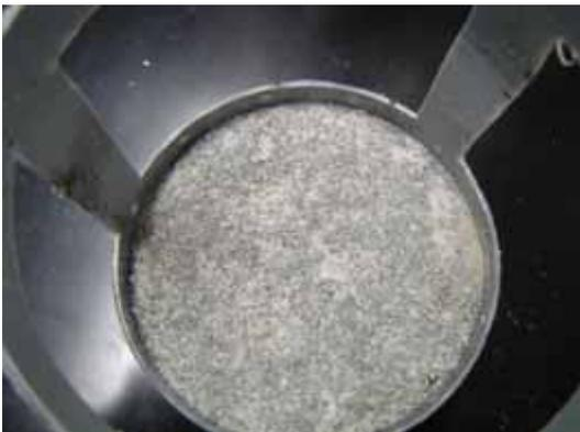
Figure 8. Less than 2 mm graded LFC material after exposure to 10 F/T cycles and flow around leaching for 21 days (note consolidation of the material).
