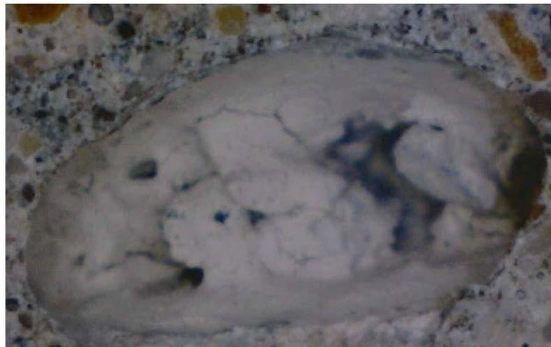
Figure 57: IL1-2 Void filled with ASR Gel
