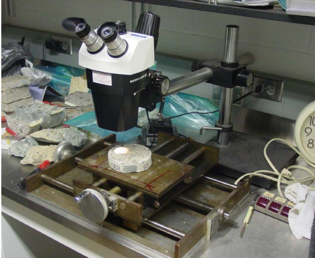
Figure 35: Olympus® SZH10 Stereo Microscope used for Petrographic Study
