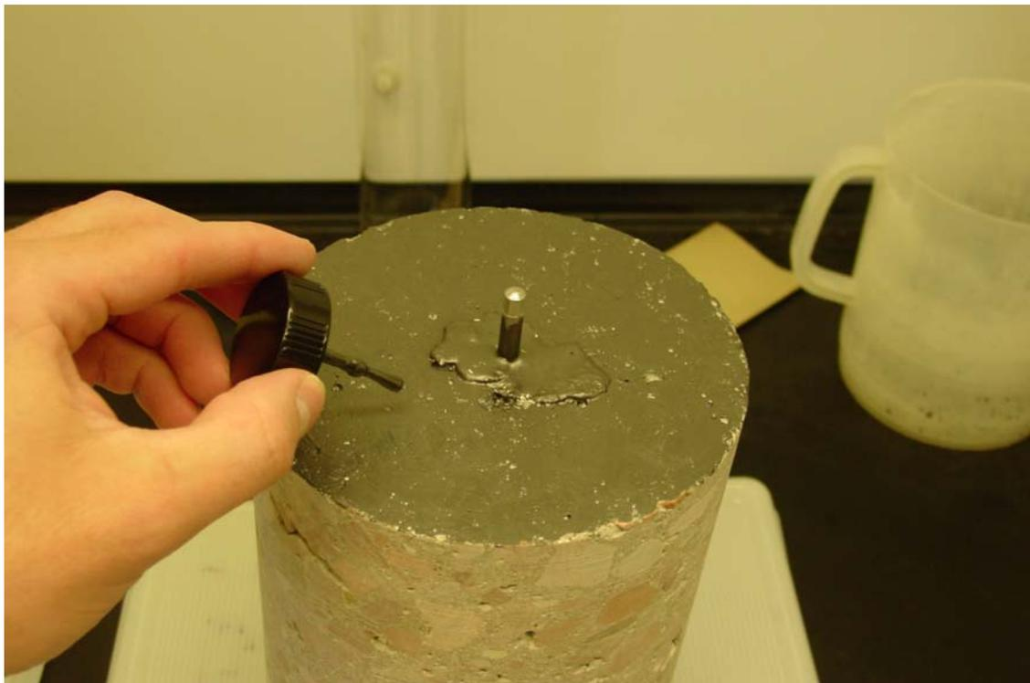
Figure 26: Core with Conductive Carbon Paint
