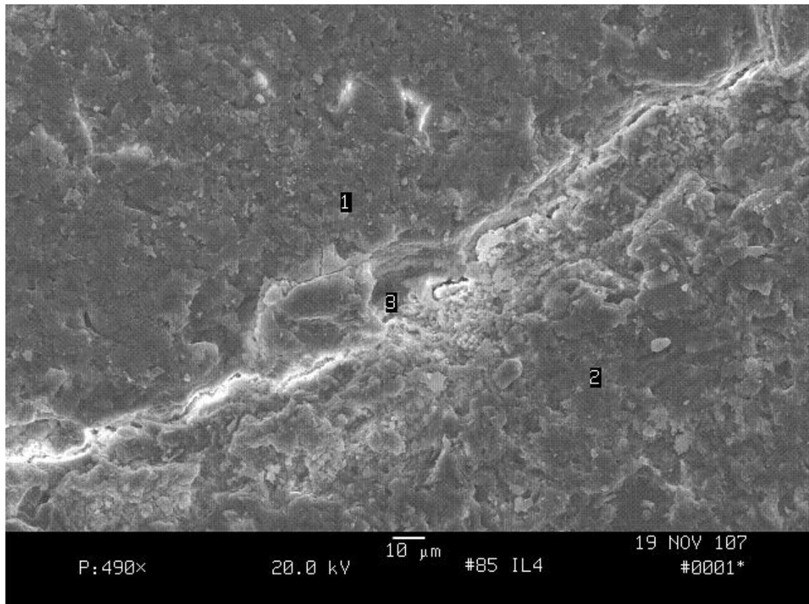
Figure 58: SEM Interpretation of Surface around Crack (IL1-1)
