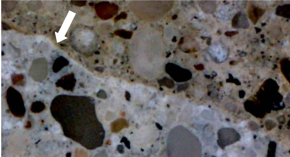
Figure 50: W11-2 RCA Border with ASR Gel Deposit
