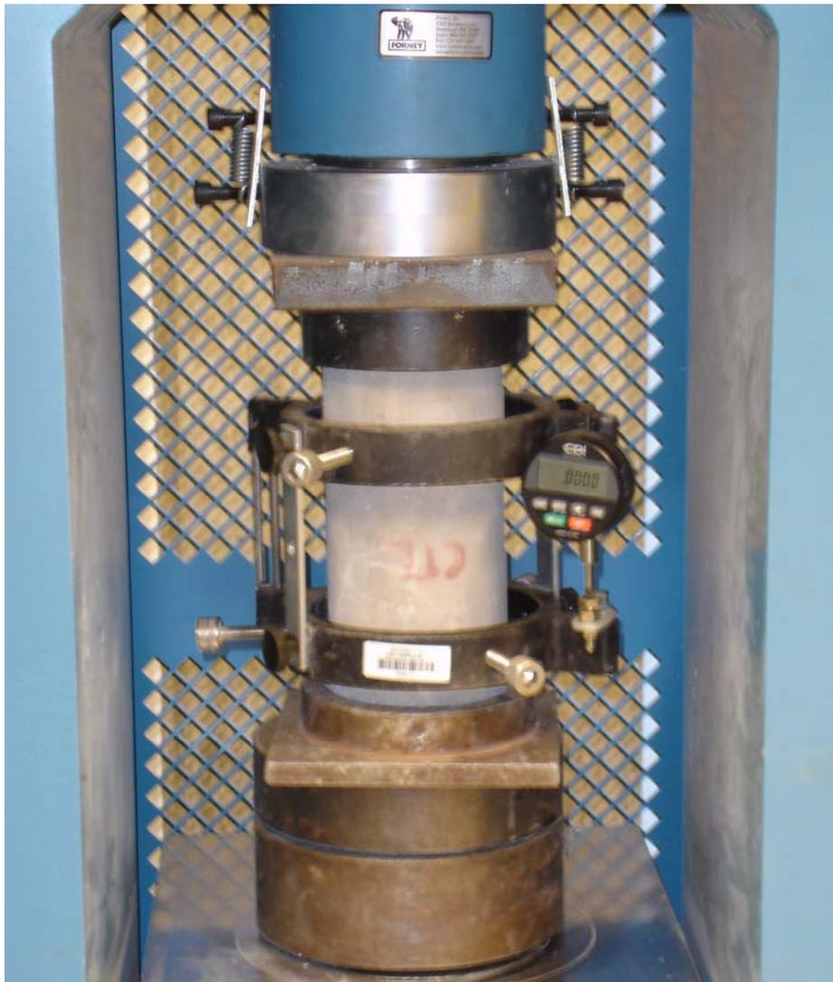
Figure 31: Core set up for Young's Modulus Testing
