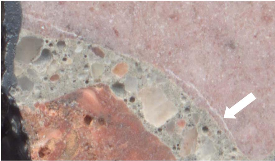
Figure 44: Typical WY1-2 (Control) Aggregate Crack with ASR Gel Deposit
