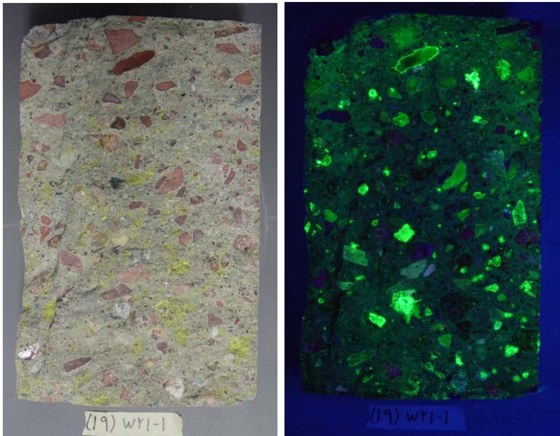
Figure 43: Fractured Core from WY recycled coated with Uranyl Acetate Dihydrate under UV light (right) showing ASR gel and under regular light (left)
