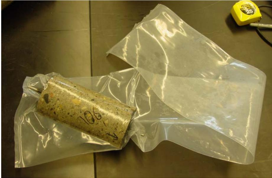
Figure 28: Vacuum Saturated Core
