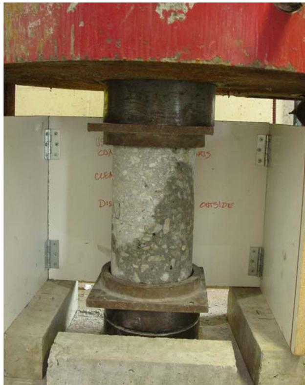
Figure 22: Core set up for Compression Testing
