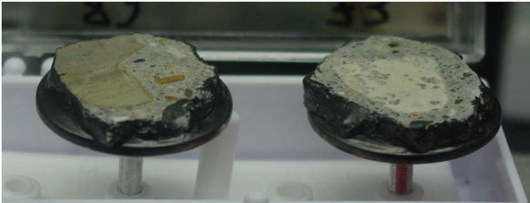
Figure 38: SEM Stubs with Affixed Concrete Specimens
