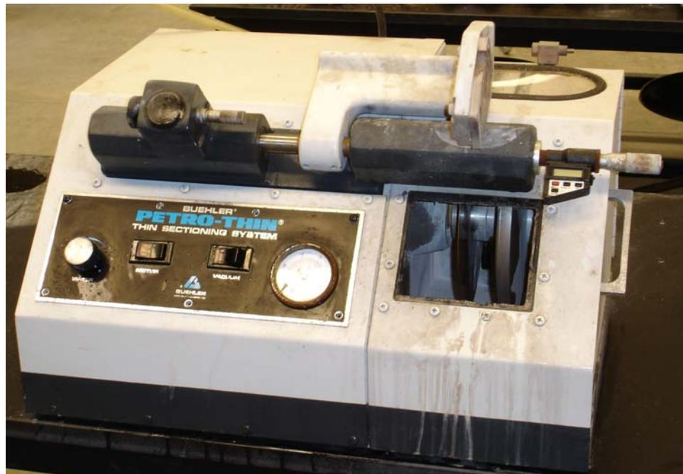
Figure 37: Buehler® Thin Sectioning Machine
