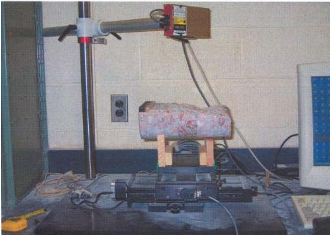
Figure 32: Volumetric Surface Texture Test Setup<sup>22</sup>
