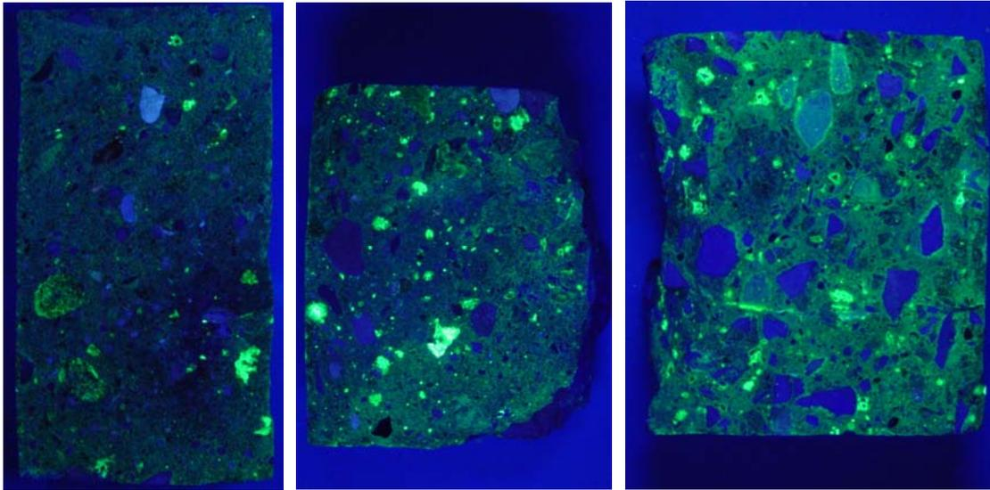
Figure 23: Uranyl Acetate Rating System, Low (left), Medium (center) and High (right)
