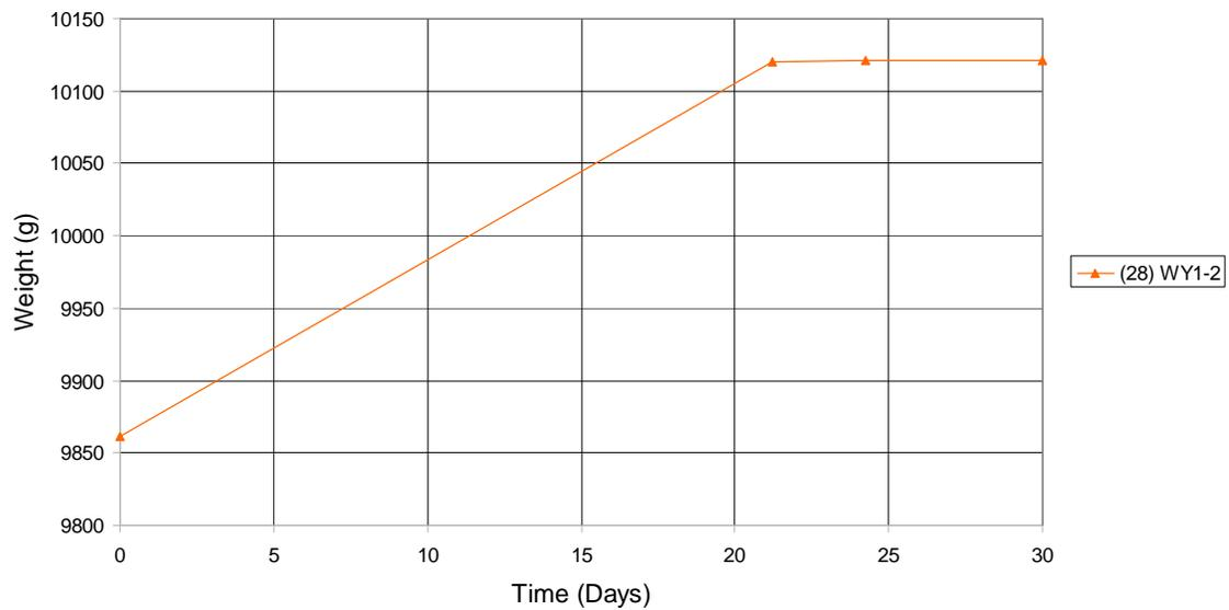
Once time vs. expansion and weight gain became asymptotic it was assumed that saturation was attained. A core under vacuum is shown in Figure 28. After the cores were determined to be at a constant moisture they were stripped from the vacuum sealed bags and their lengths and weights were recorded.
