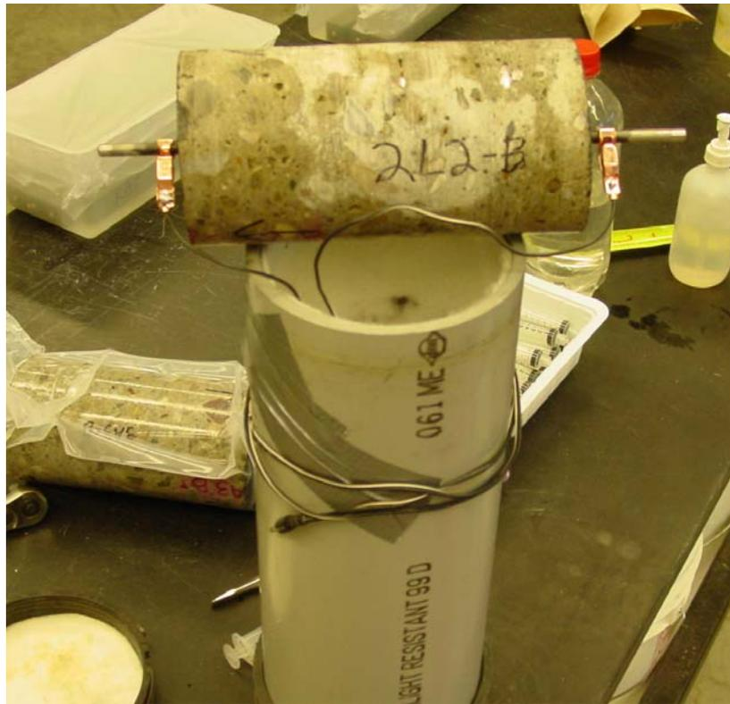
Figure 29: Modified ASTM C 1293 (Electric Cylinder) Test Setup
