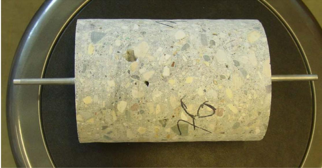
Figure 25: Studded Core for Modified ASTM C 1293 Testing
