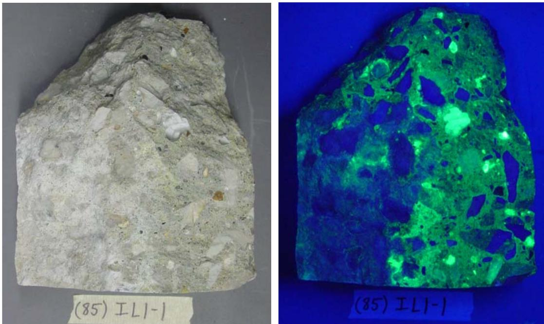
Figure 53: Fractured Core 85 (IL 1-1) coated with Uranyl Acetate Dihydrate under UV light (right) showing ASR gel and under regular light (left)
