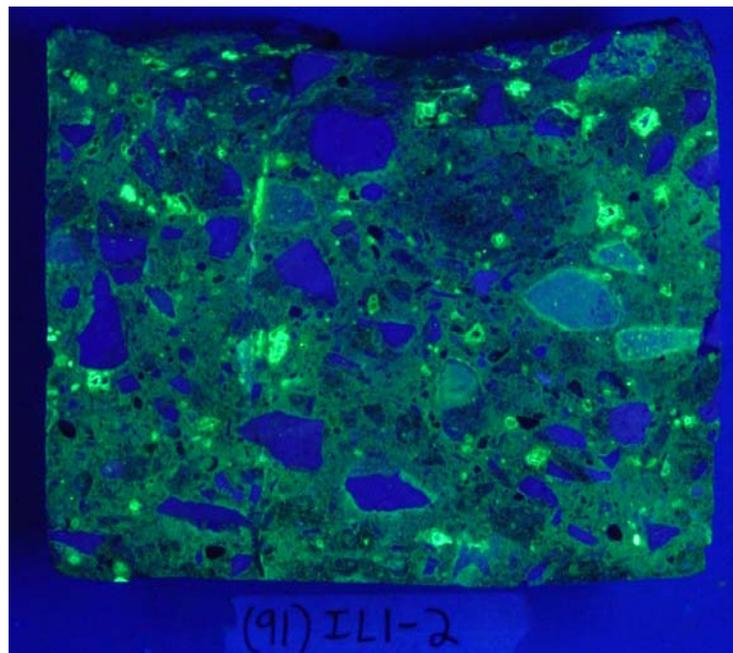
Figure 55: Fractured Core 91 (IL 1-2) coated with Uranyl Acetate Dihydrate under UV light
