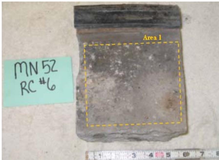
Figure 33: Typical Joint Face Area used for VST Testing<sup>22</sup>
