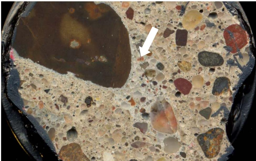
Figure 51: W11-1 Crack Propagating from RCA
