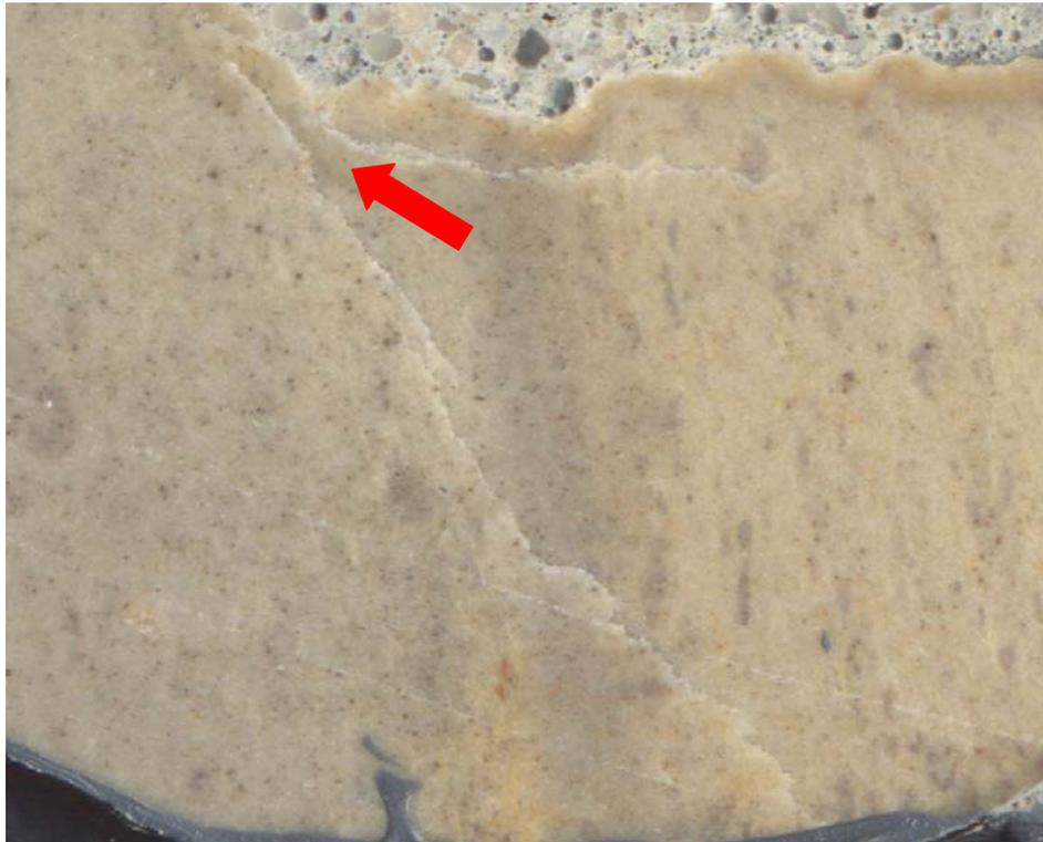
Figure 52: W12-2 Aggregate Crack with ASR Gel Deposit
