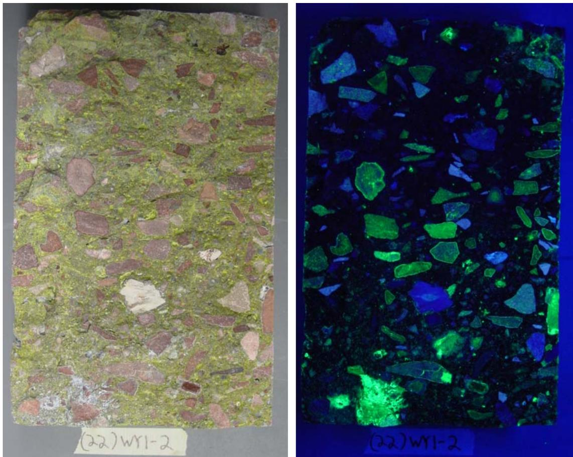
Figure 42: Fractured Core from WY control coated with Uranyl Acetate Dihydrate under UV light (right) showing ASR gel and under regular light (left)
