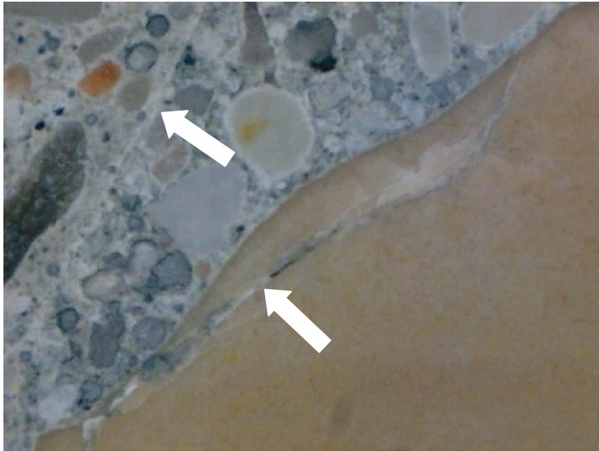
Figure 45: WY1-1 (Recycled) Aggregate Crack and RCA border with ASR Gel Deposits
