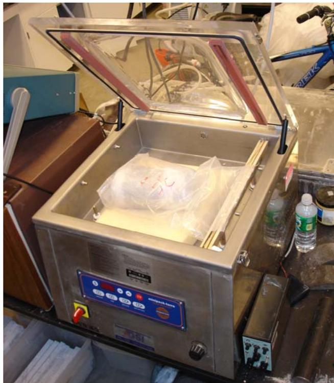
Figure 18: Core in Vacuum Sealing Machine
