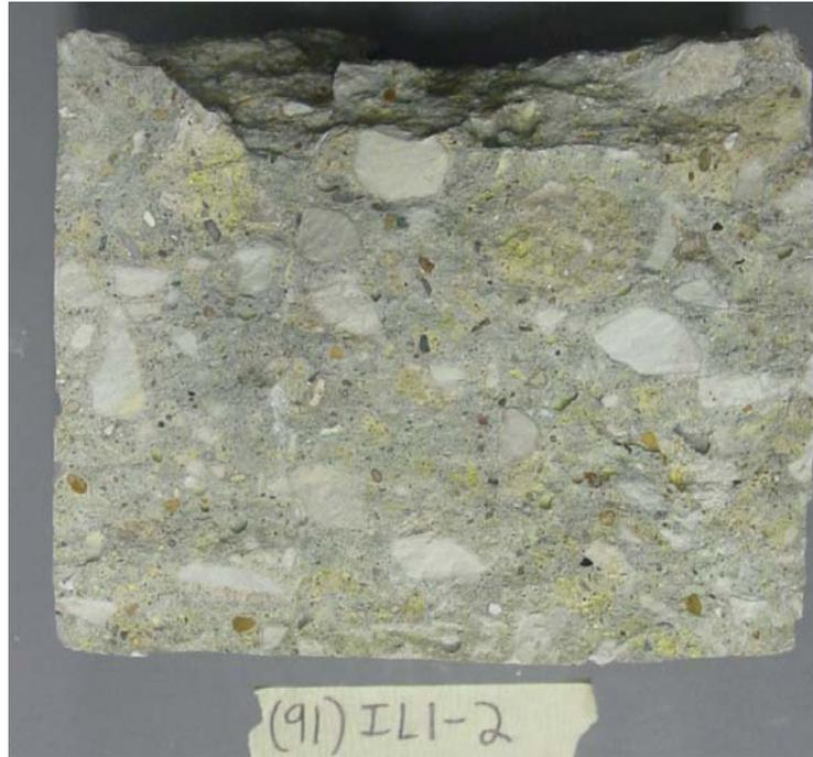
Figure 54: Fractured Core 91 (IL 1-2) coated with Uranyl Acetate Dihydrate under regular light
