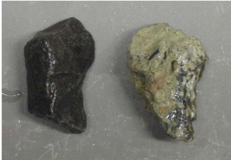
Figure 1: Original Aggregate (left) and Recycled Concrete Aggregate (right)
