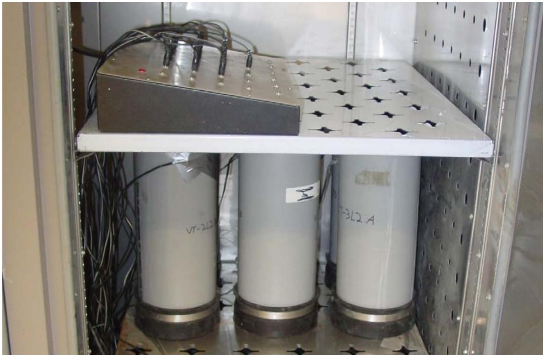
Figure 30: Modified ASTM C 1293 Core Storage Containers in Oven
