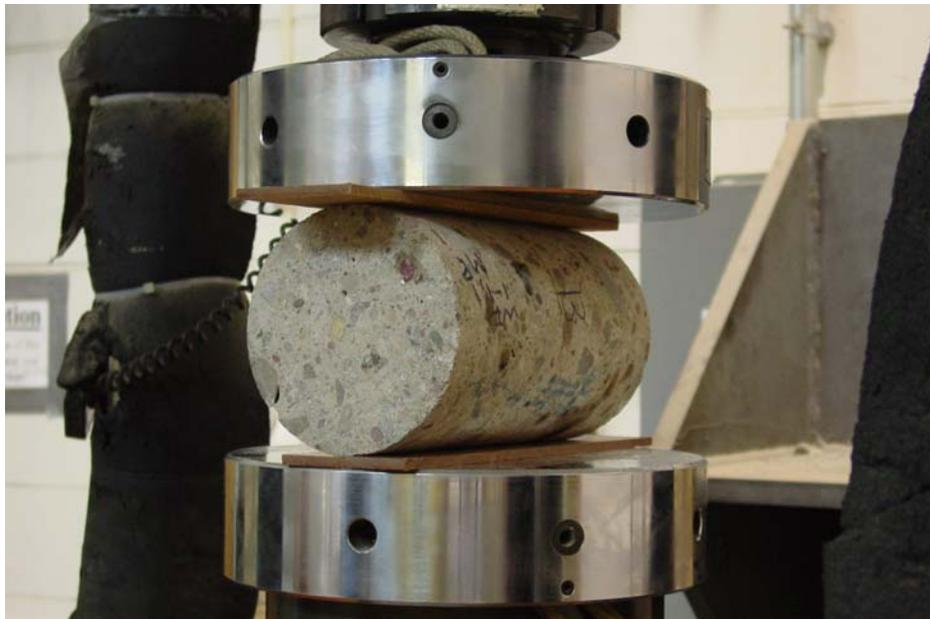
Figure 19: Core set up for Splitting Tensile Strength Testing
