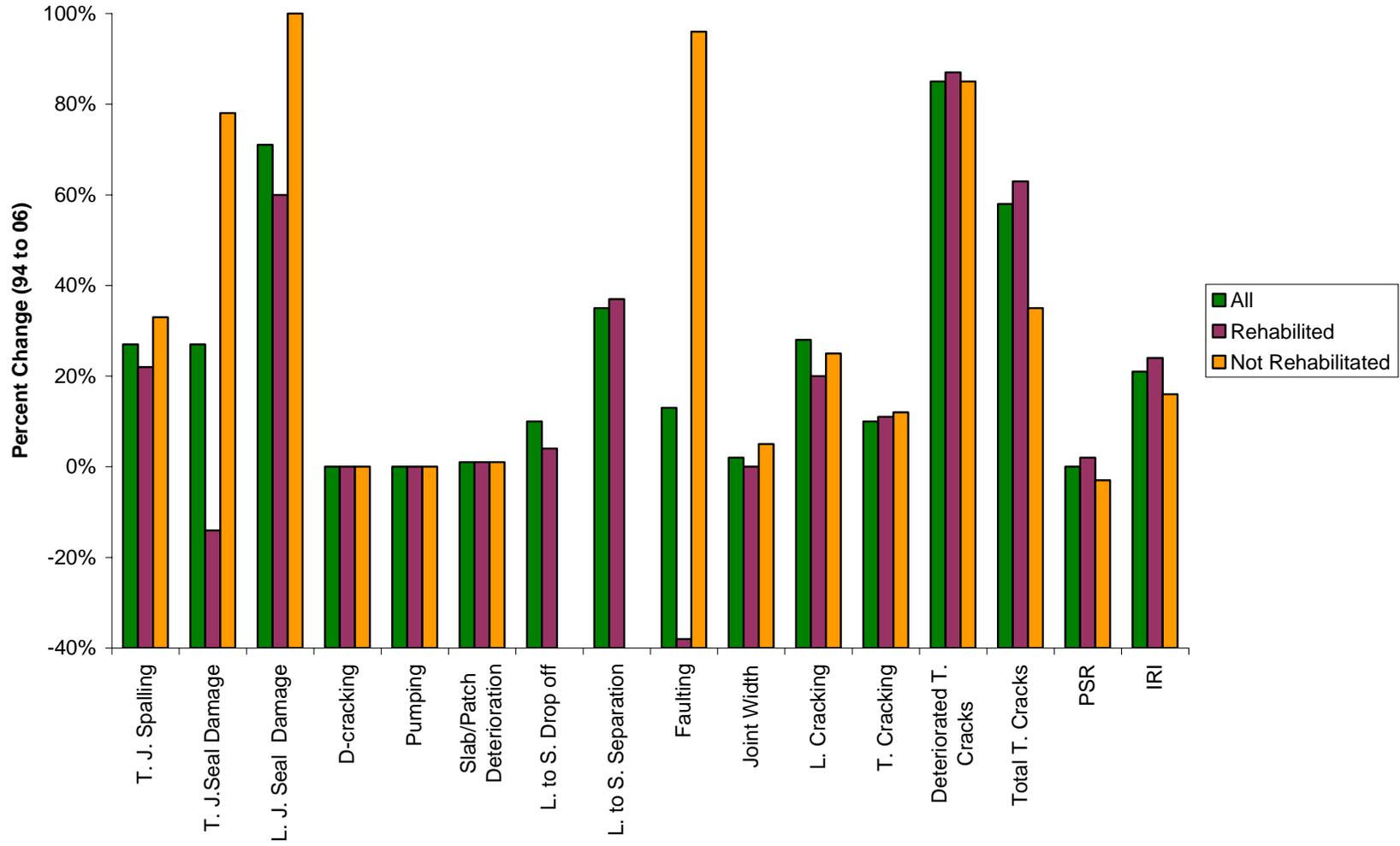
Figure 60: Control Pavement Distresses (Avg. Percent Change from 1994 to 2006)
