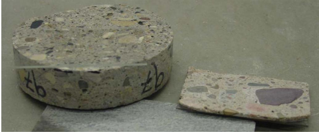
Figure 36: Original Core Cap and Thin Section Epoxy to Glass Slide
