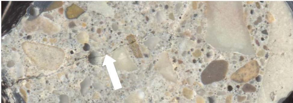
Figure 56: IL1-1 Crack Propagating from RCA
