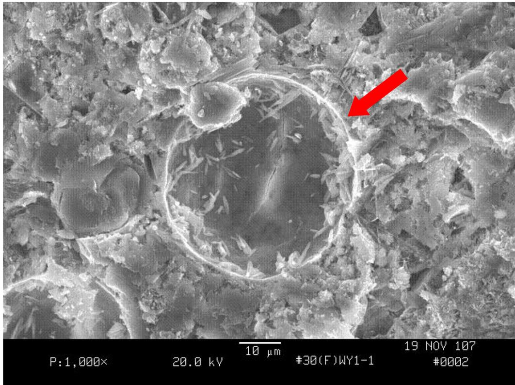
Figure 47: SEM Interpretation of a Fly Ash Particle's Surface (WY1-1)
