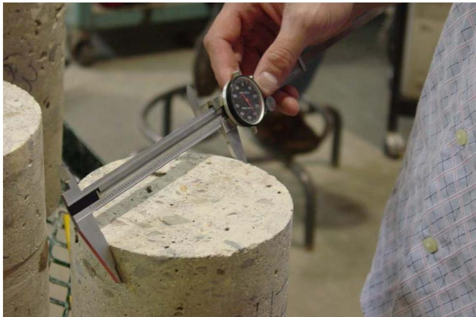
Figure 21: Measuring the Diameter of a Cylinder with a Caliper
