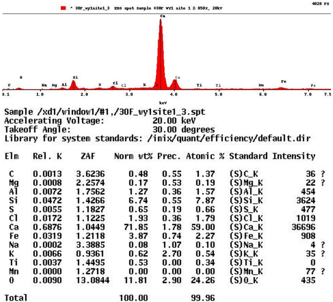
Figure 46: Elemental Analysis showing high Calcium Content
