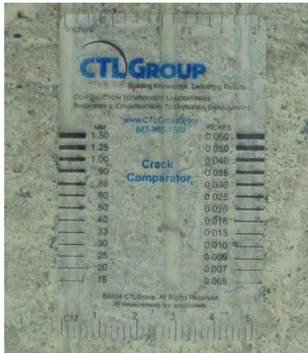
Figure 8: Crack Comparator Card
