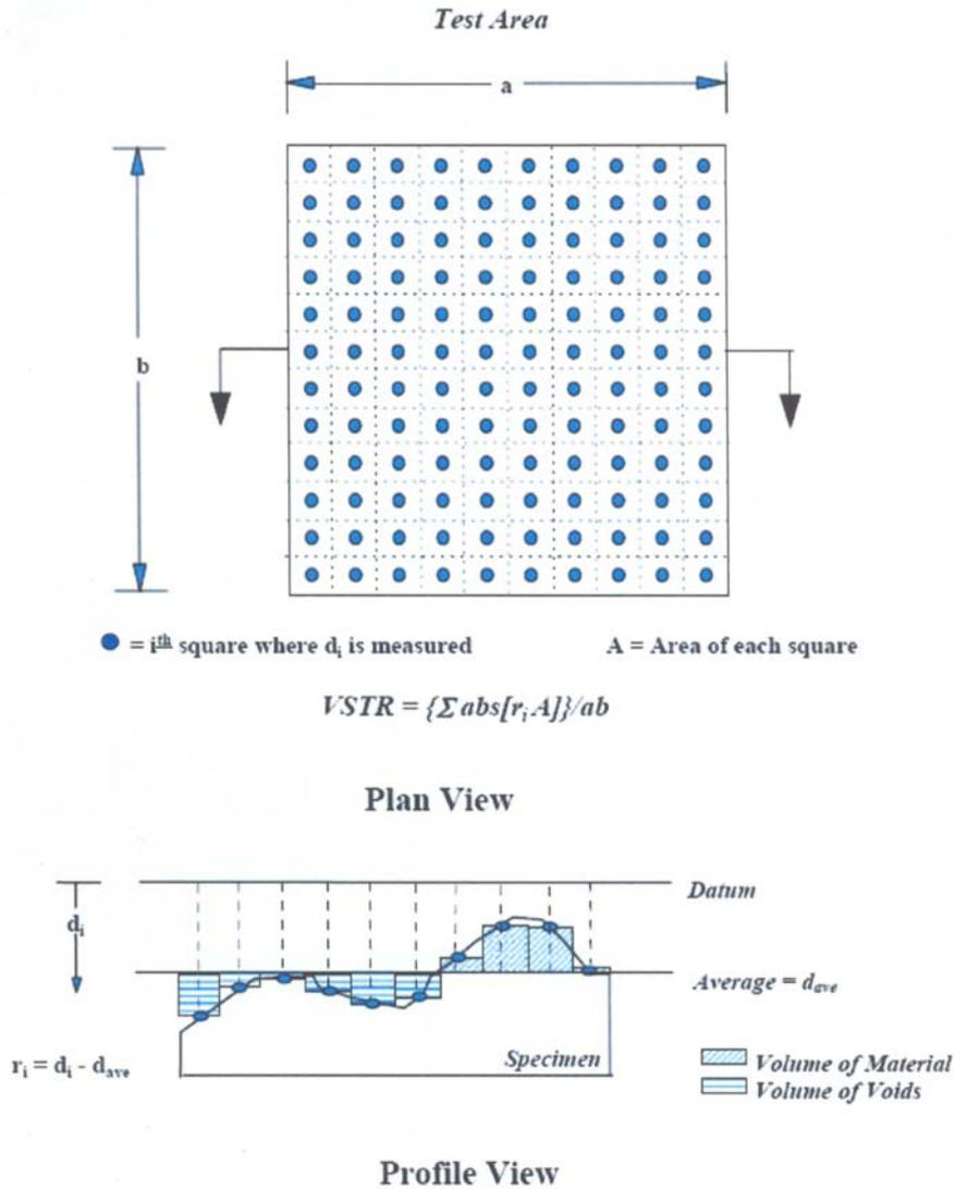
Figure 34: Graphical Representation for VST Calculations<sup>22</sup>
