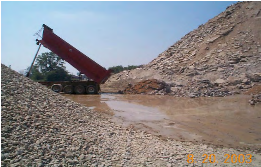
Figure 7. Truck unloading concrete debris. Iafrate Crushing Plant Visit. Taylor, MI
