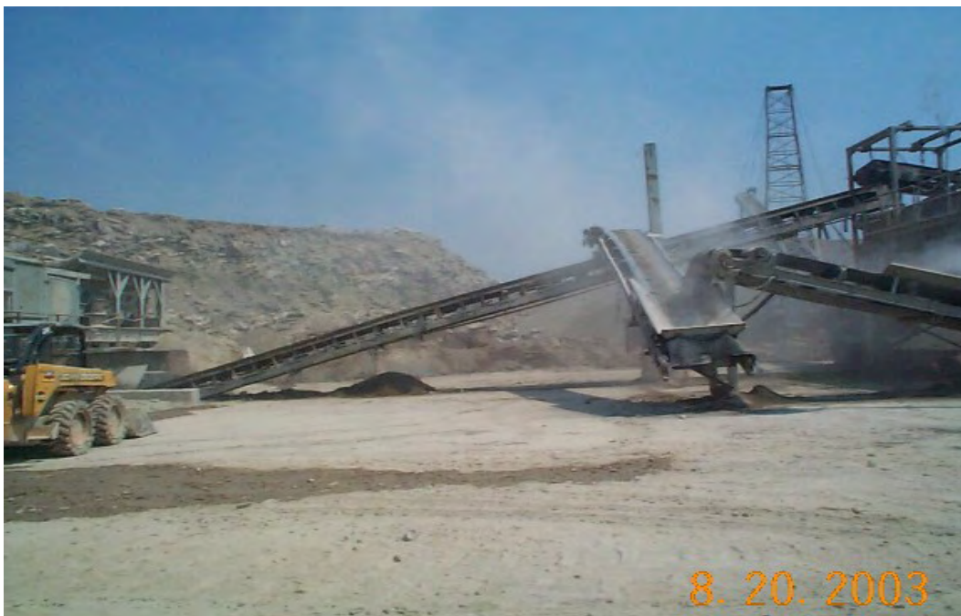
Figure 10. Vibrating-feeder transporting RCA from Primary Crusher to sorting screen. Iafrate Crushing Plant Visit. Taylor, MI
