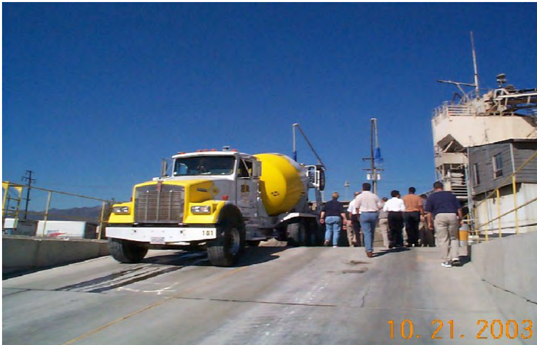
Figure 21. Truck Dumping Plastic Portland Cement Concrete (PPCC) to the Reclaim System. Red-I-Mix Concrete Inc. Facility Visit. Irwindale, CA
