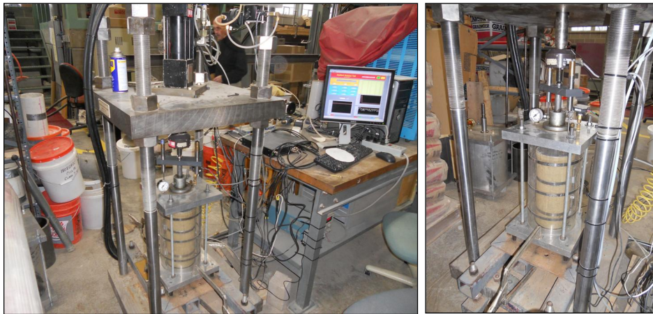
Figure B-3 Photo of the Repeated Loading Machine Illustrating the Resilient Modulus Test (from the UW-Madison, USA)
