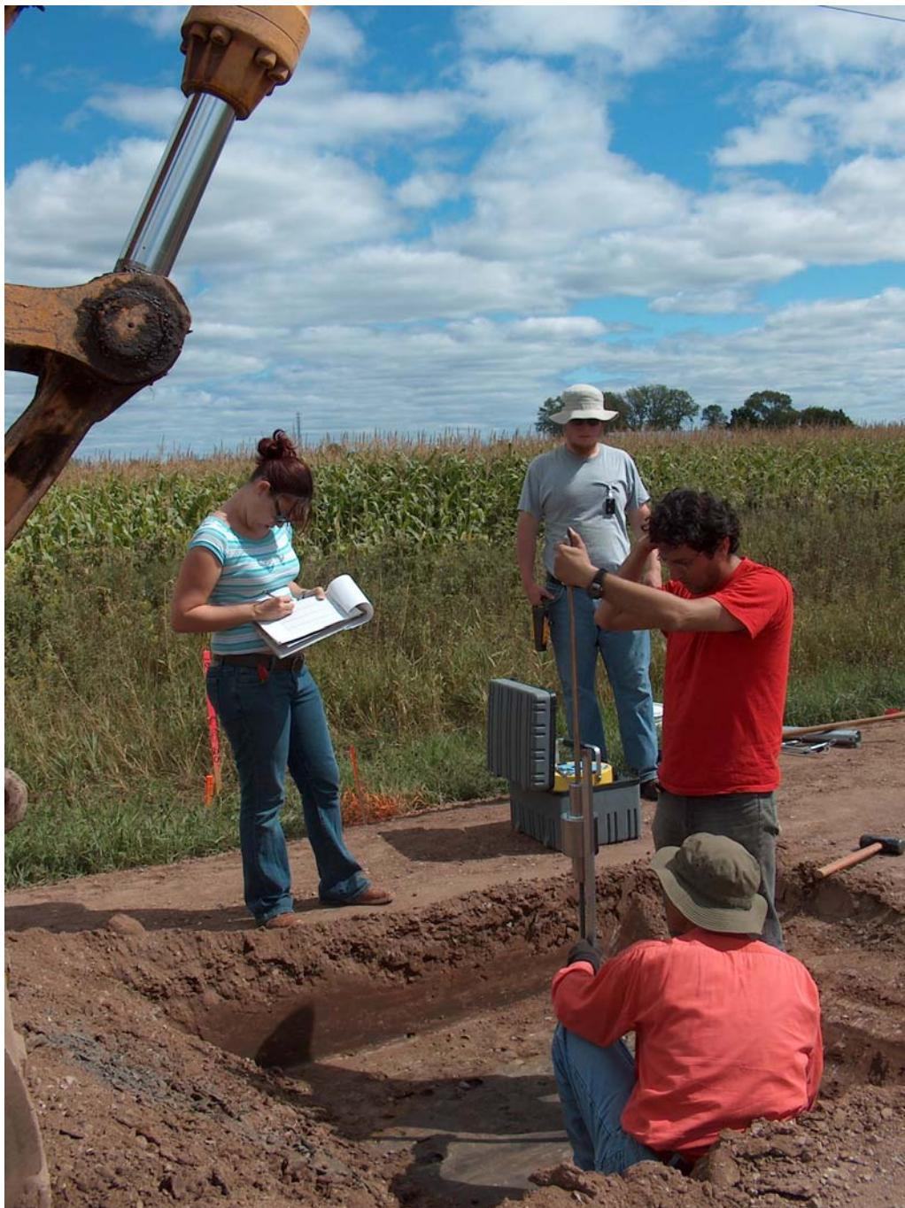
Fig A4. Dynamic cone penetration (DCP) test on subgrade
