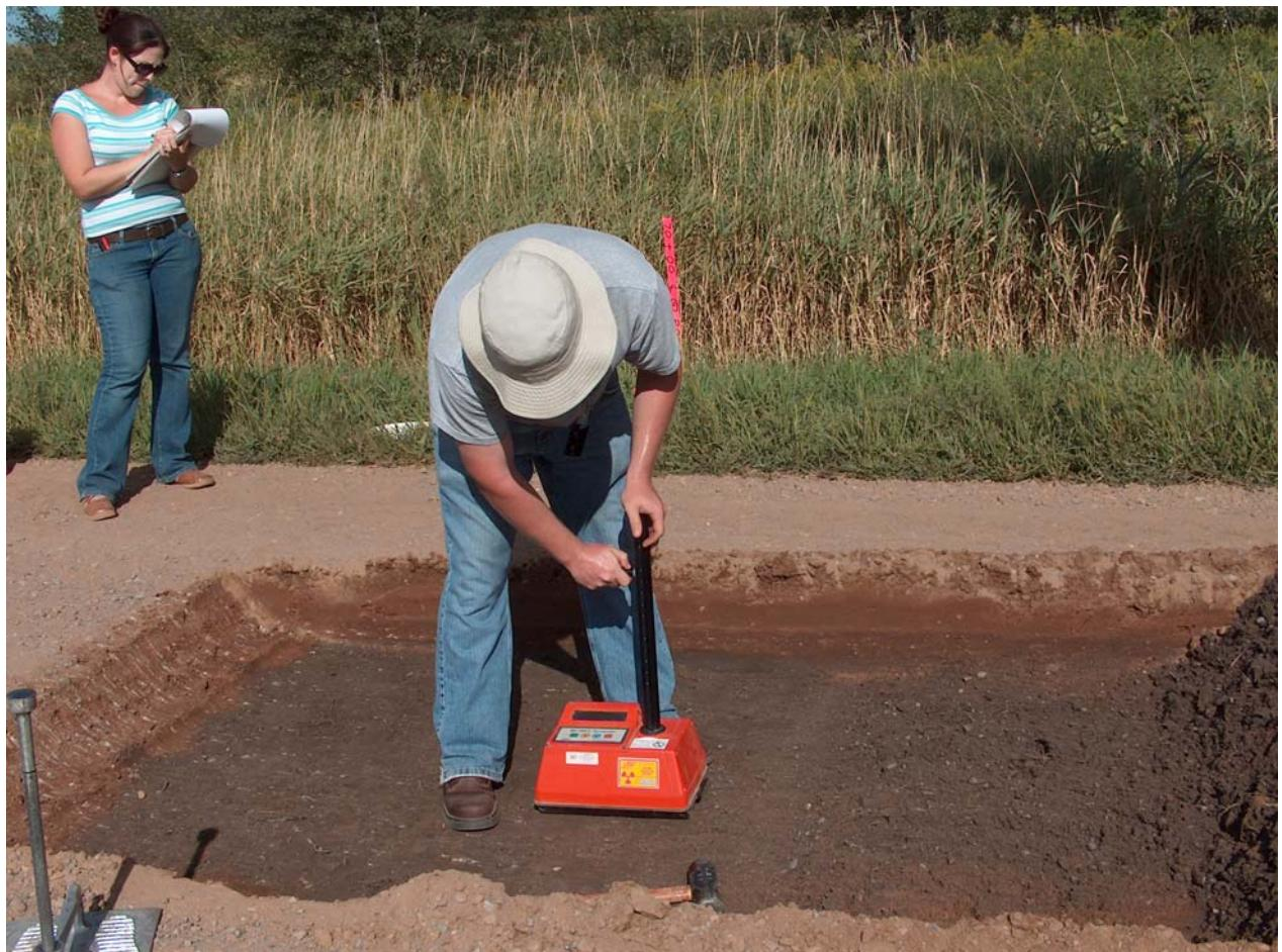
Fig A3. Measurement of water content and unit weight of subgarde.
