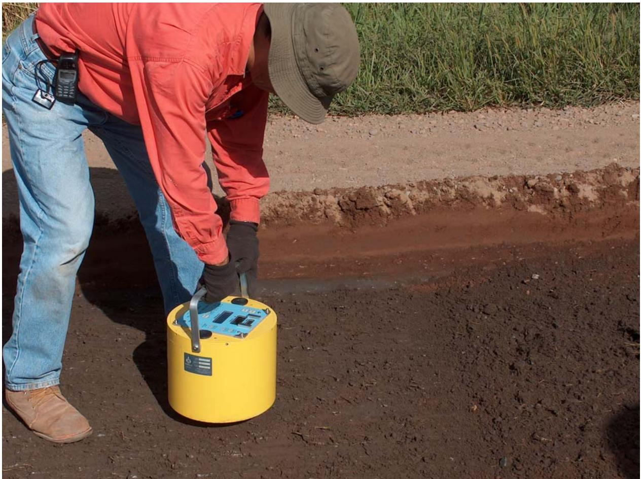
Fig A2. Soil Stiffness measurement by using SSG on subgrade.
