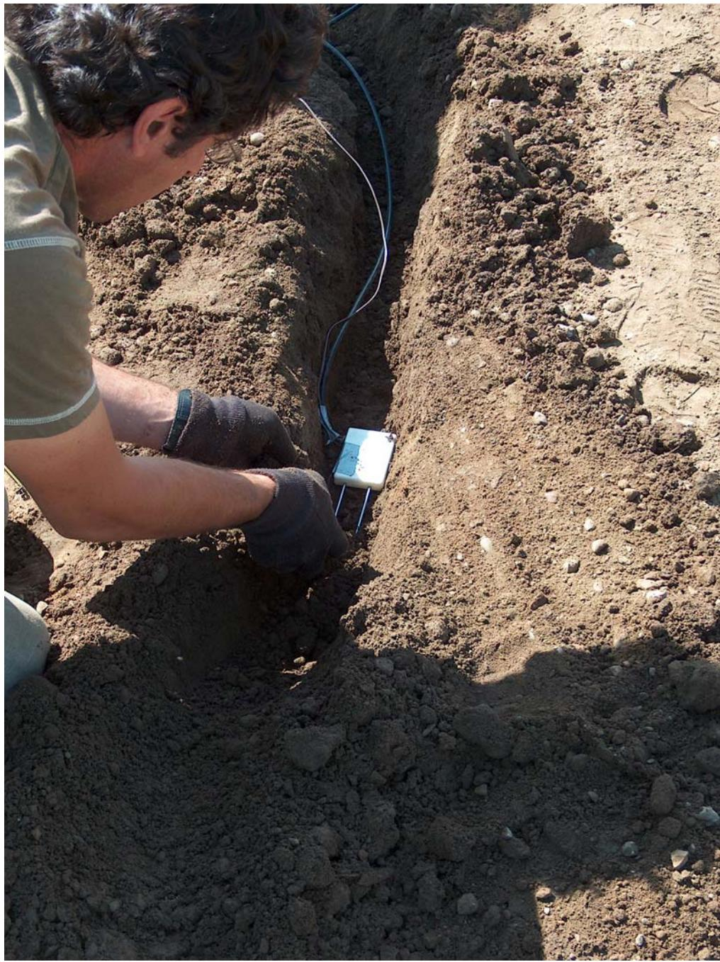
Fig A20. Installation of volumetric water content and temperature sensors (Sensor 3) into S-RSG on lysimeter.
