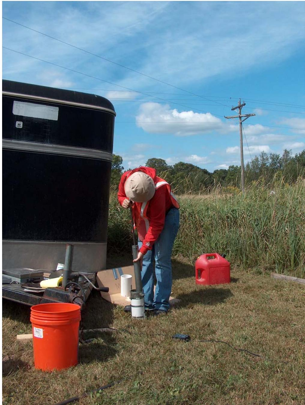
Fig A13. M<sub>r</sub> and CBR sample preparation of field mix soils collected with in 1-2 hour of blending process.
