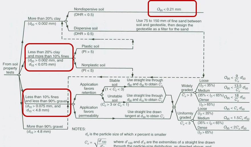
through the particle-size distribution, as directed above; and  $d'_{50}$  is the midpoint of this line.
