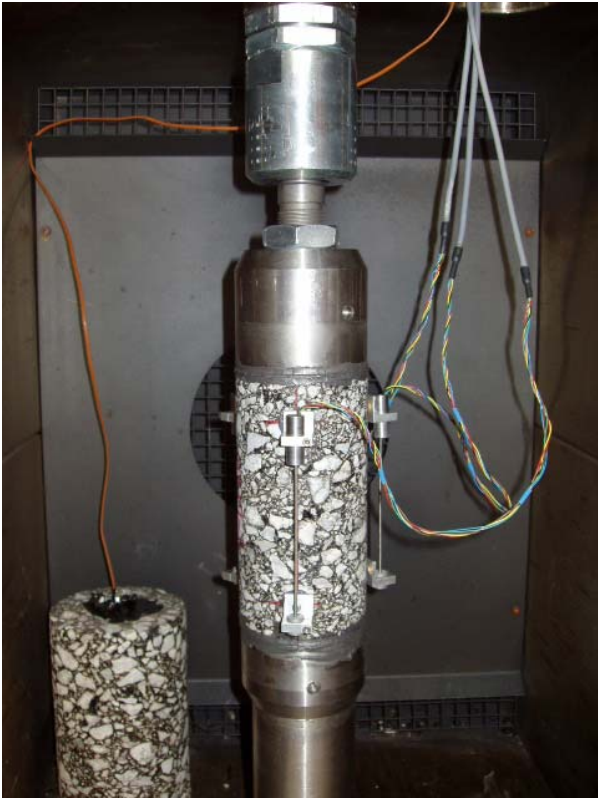
FIGURE 2 Test Setup (a) Compression (b) Tension
