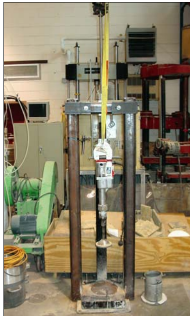
Demolition hammer used for vibratory compaction of granular aggregates.
