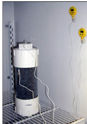
One of the 250 mm long columns used for the leaching experiments.
