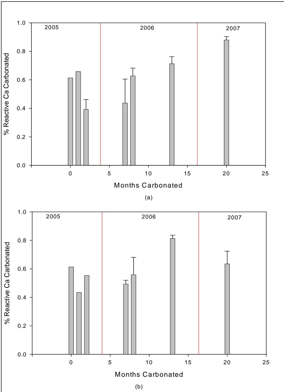
**Figure 7.1 – Observed Percent Calcium Carbonation Concentrations in Pile A over 20 Months**
