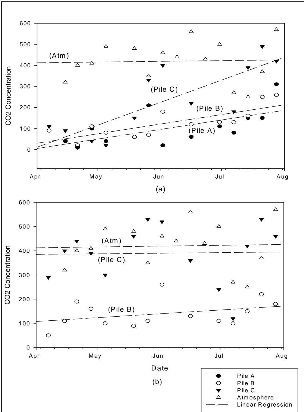
**Figure 7.4 – Weekly CO<sub>2</sub> Concentrations within Piles A, B and C with Linear Regression**
