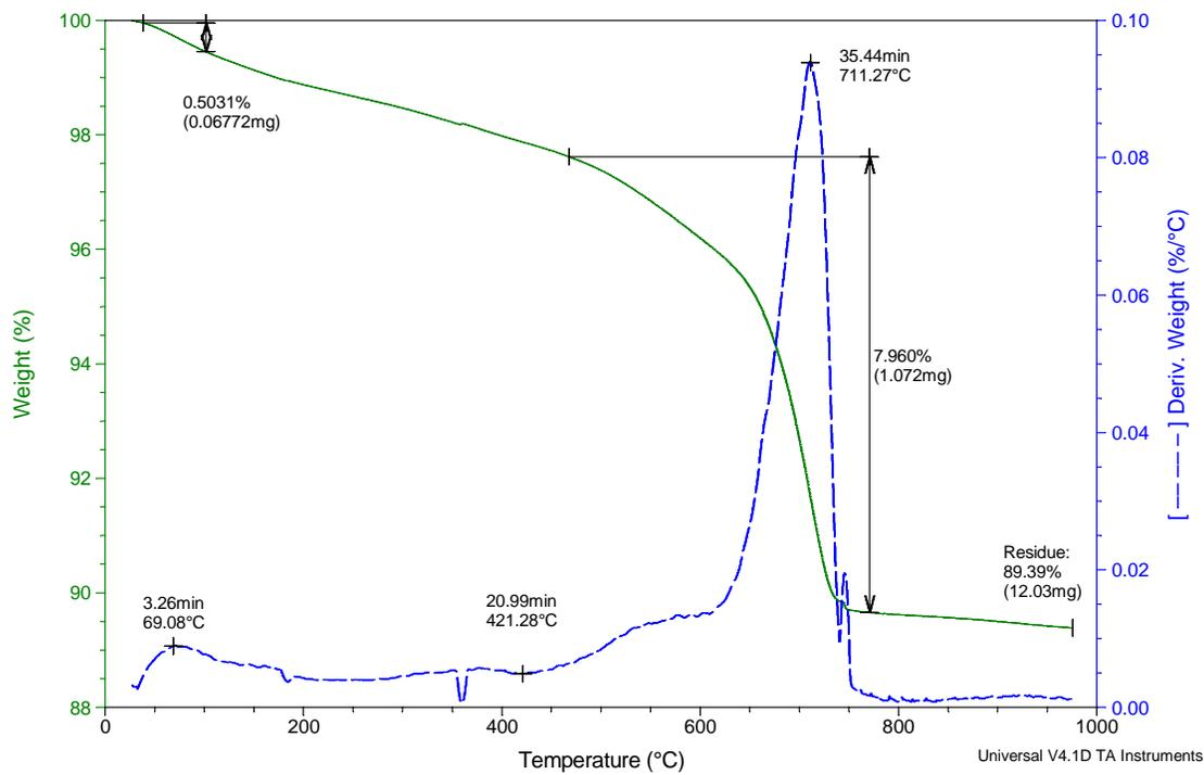
Figure 9 TGA Curve of RCF-49
