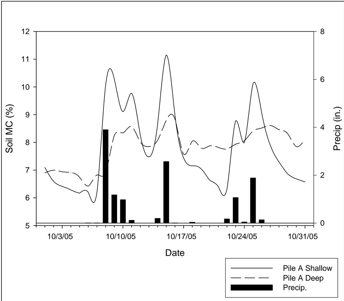
Figure 7.7 – Moisture Content of Pile A in Conjunction with Rain Events between in October, 2005
