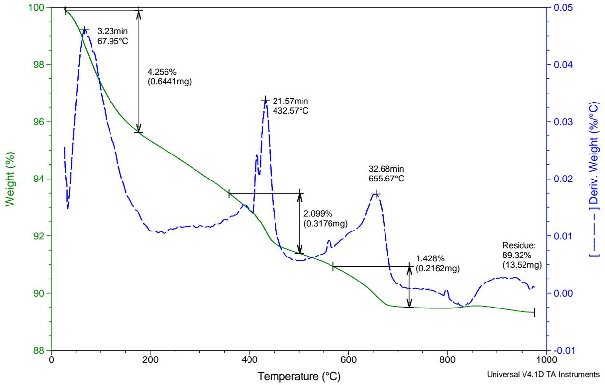
Figure 13 TGA Curve of SLC-RCF
