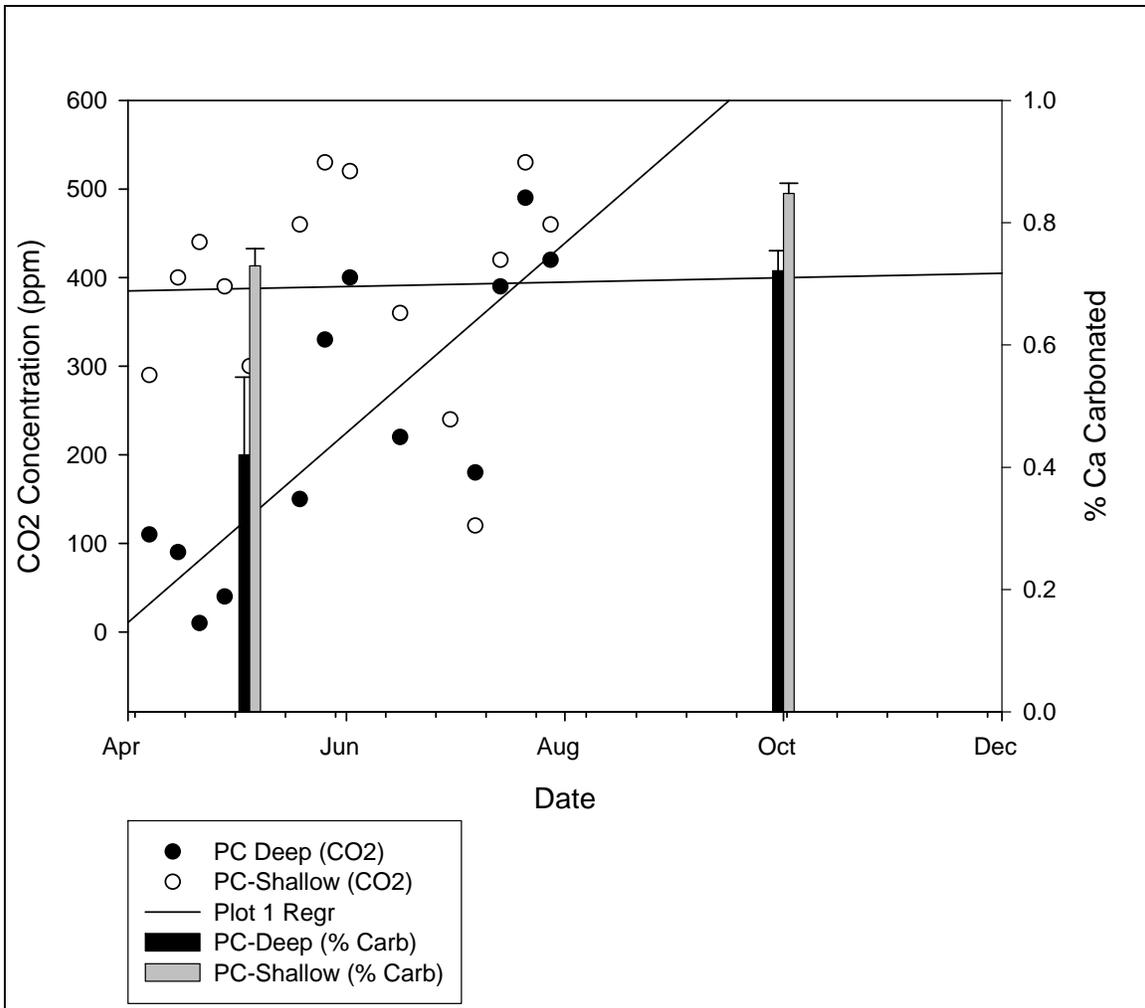
**Figure 7.5 - TGA and CO<sub>2</sub> Concentrations of Pile C between April and October of 2006**
