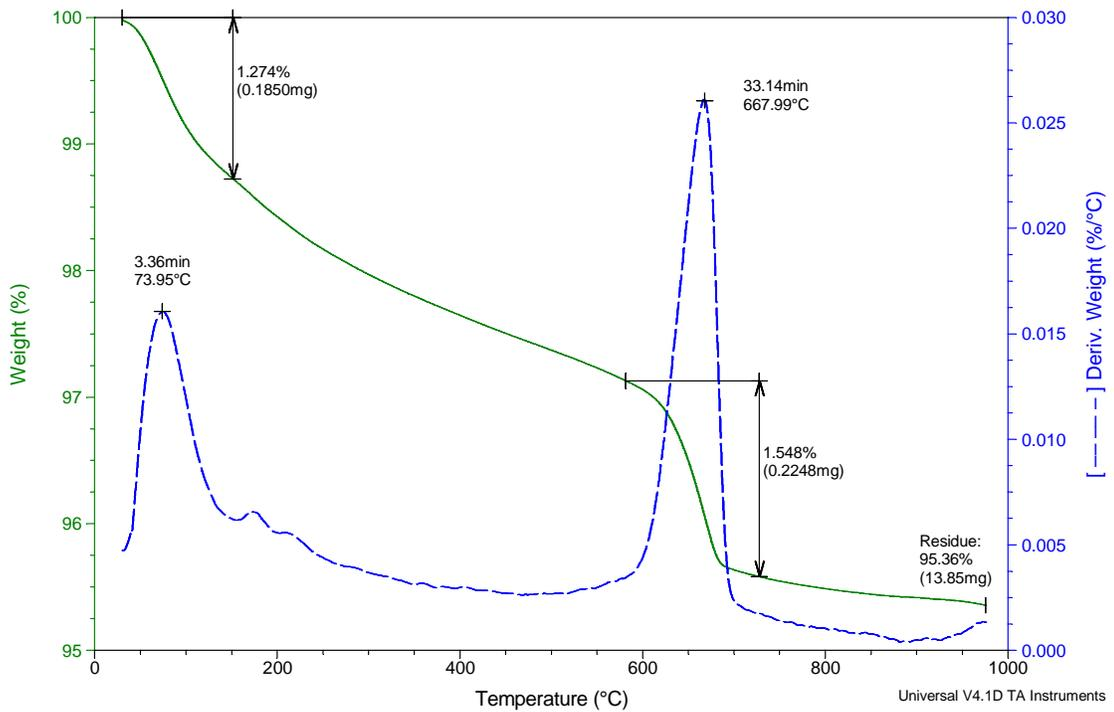
Figure 1 TGA Curve of CFA-7
