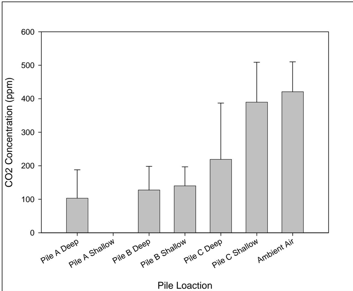
**Figure 7.3 – Average Carbon Dioxide Concentrations within Piles A, B,C and the Ambient Air**
