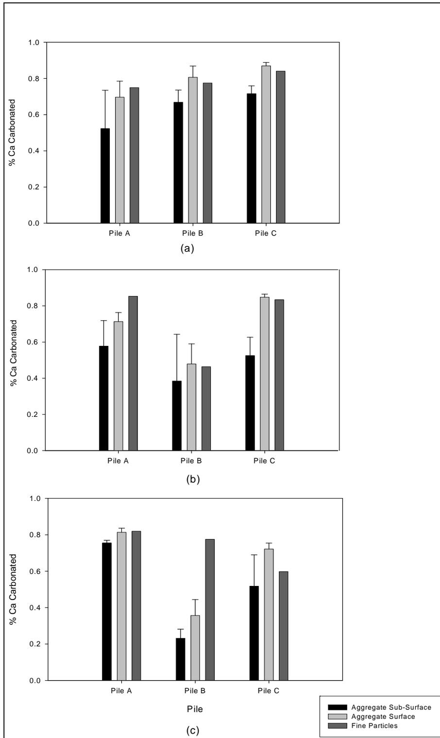
**Figure 7.2 – Observed Percent of Rective Ca Carbonated at 13 Months**
