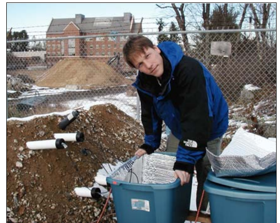
RMRC researcher Scott Greenwood collecting data from instrumented piles of recycled concrete material behind UNH's Gregg Hall.
