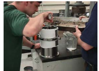
Filling the slotted mold with sample material for compacting.
