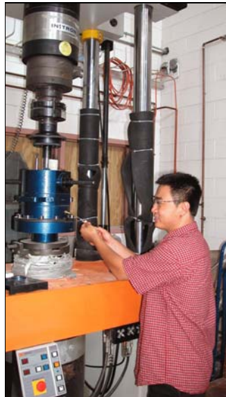
Graduate student Xinghe Li uses a pore water extraction device to test samples of recycled concrete aggregate (RCA) and standard concrete samples.
